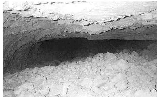
The broken rock pile is spread relatively evenly between the face and the barricade with a wide range of size distribution.
