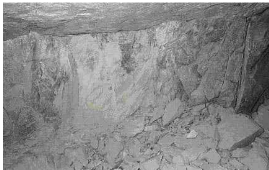
No sockets left on the face after the blast using MYDO Sonic Tamping Lock Plugs and Magnum 365 explosive. A coarse fragmentation overall, with relatively no broken rock in the first metre from the face.
