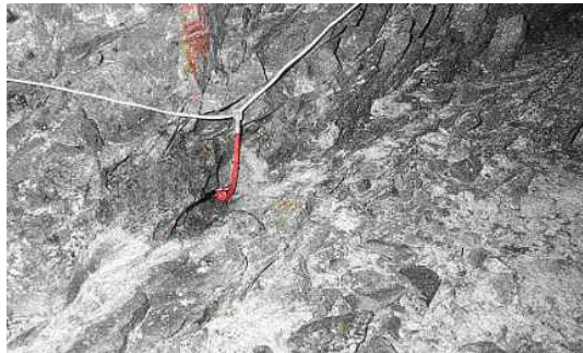
The red point of the MYDO Sonic Tamping Lock Plug, visible in the hole – just beyond the fractured zone.
